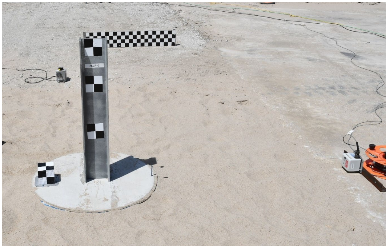
Figure 4.3 Typical String Potentiometer Setup, Test Nos. AKLP-1 and AKLP-2
