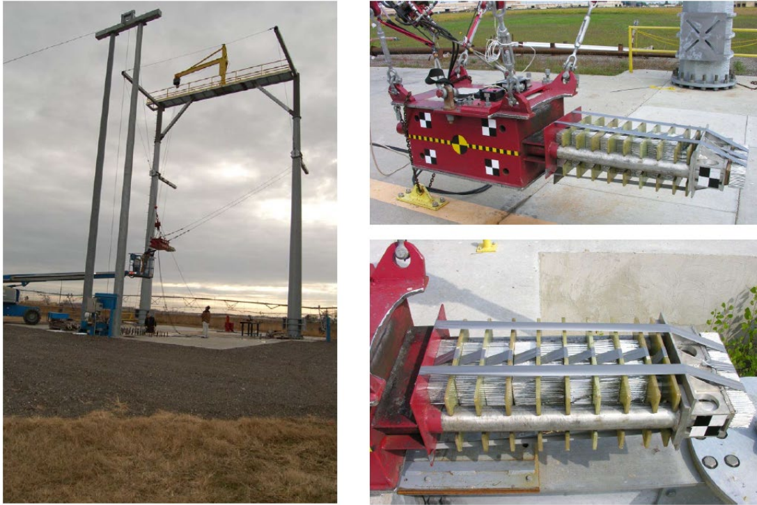
Figure 2.6 NYSDOT Aluminum Sign Testing – Pendulum and Crushable Nose [10]
