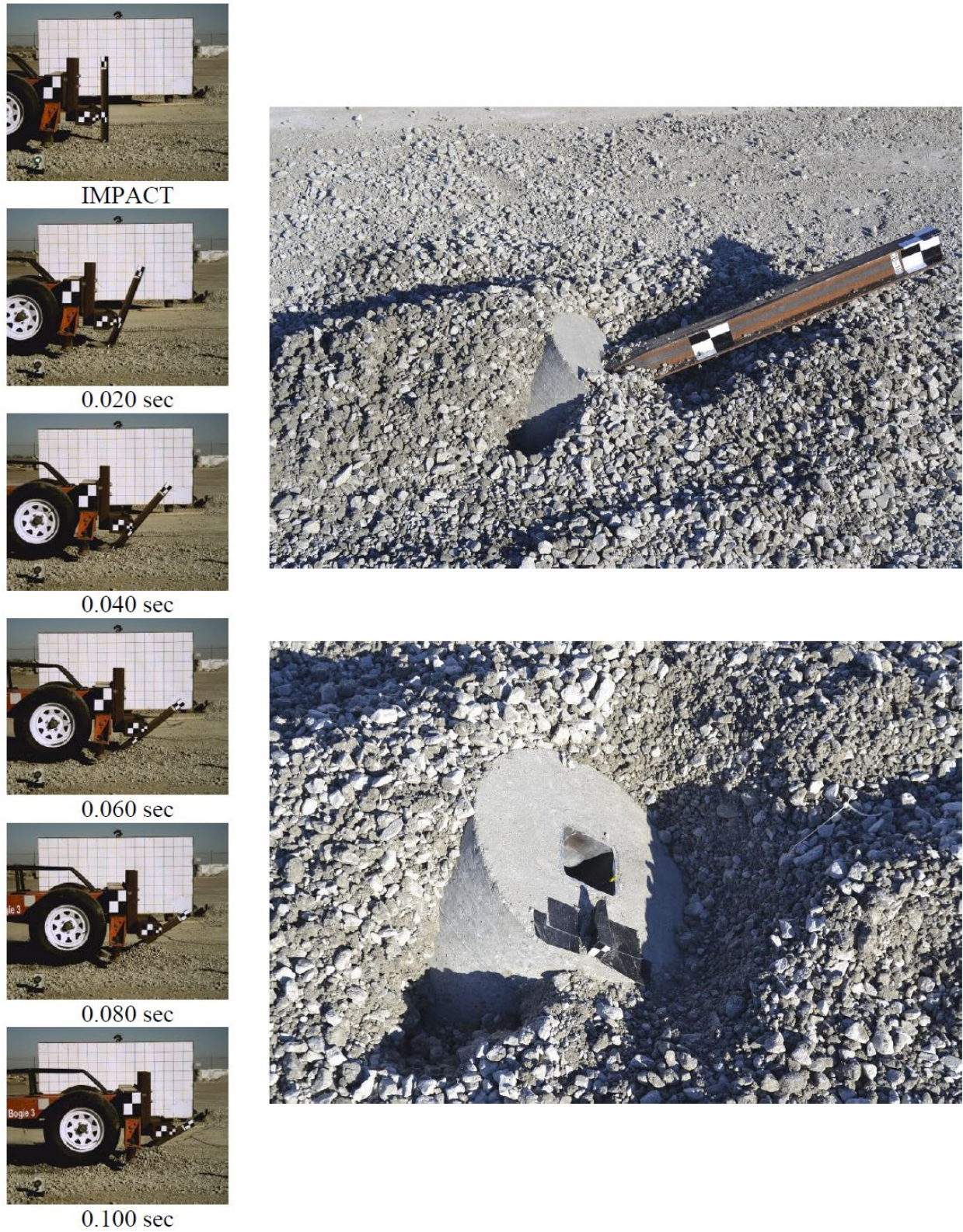
Figure 2.14 Time-Sequential and Post-Impact Photographs, Test No. HTCB-18 [15]
