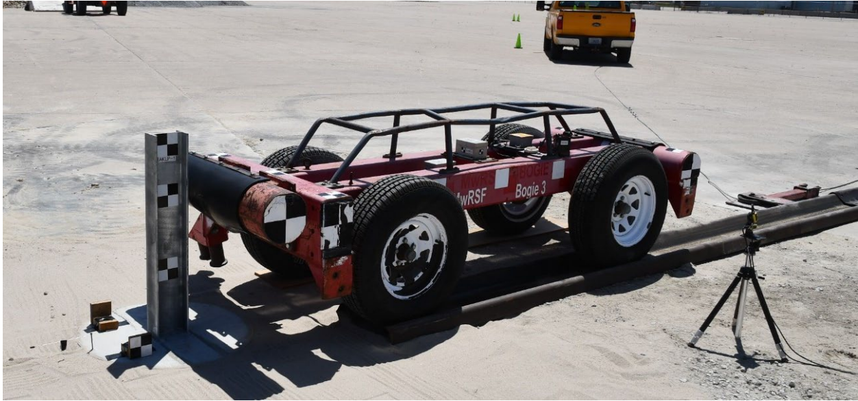
Figure 4.1 Rigid-Frame Bogie on Guidance Track Preparing to Impact Embedded Steel Post
