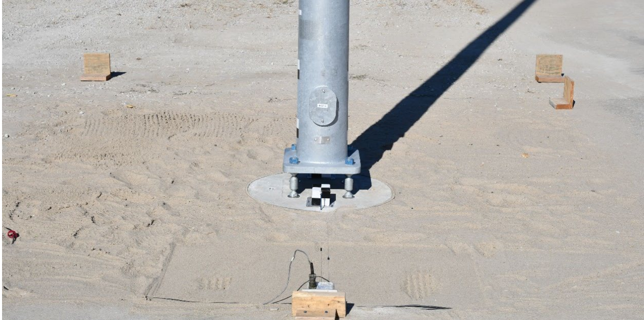
Figure 4.4 Typical String Potentiometer Setup, Test Nos. AKLP-5 and AKLP-6
