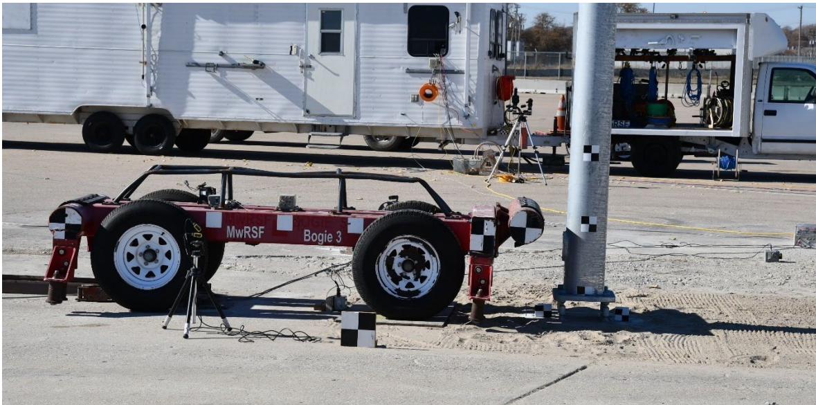
Figure 4.2 Rigid-Frame Bogie on Guidance Track Preparing to Impact Light Pole
