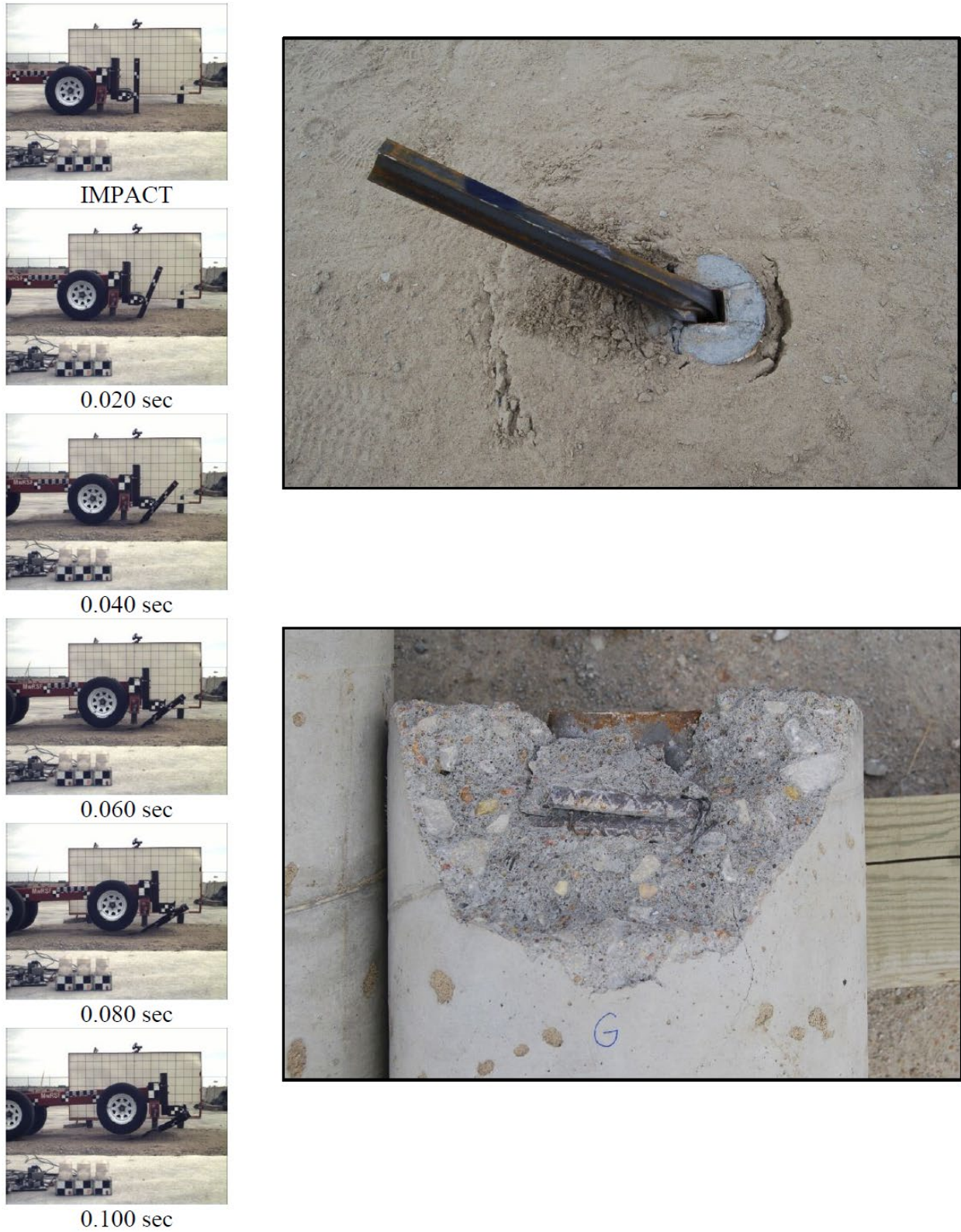
Figure 2.16 Time-Sequential and Post-Impact Photographs, Test No. HTCB-9 [15]
